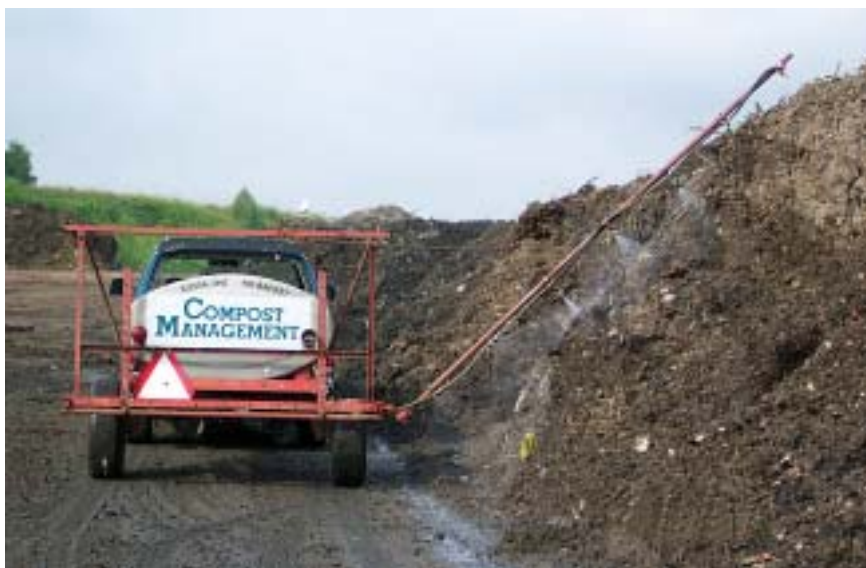
Above: Using an agricultural spray system, windrows are topically sprayed to maintain odour control.
